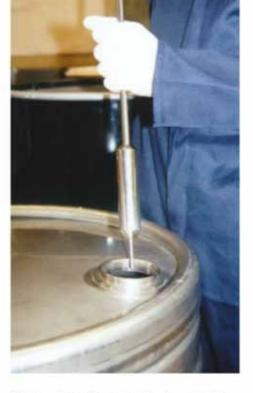
Only when the sampler is pushed against the base of the container will the sample be taken.
